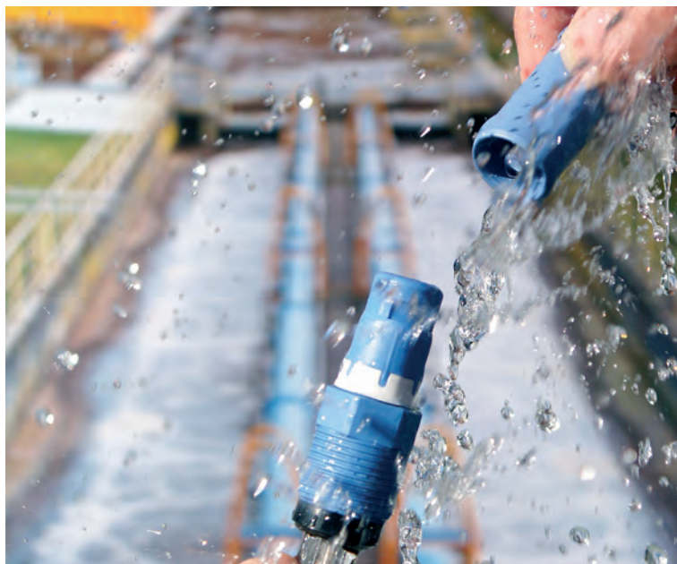
Memosens: inductive transfer of data non affected by moisture, water or corrosion
