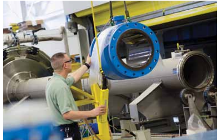
A worker hoists an electromagnetic flowmeter into position to be factory calibrated on an ISO 17025 certified calibration rig
