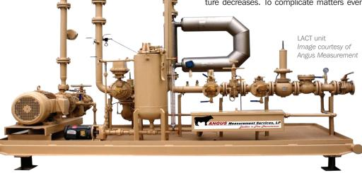
more, the volume of different crude oils change differently with temperature. The API developed tables that determine the amount of this change based on the API gravity of the crude oil. This change in volume is why the volume of the crude oil is corrected to a standard temperature, usually 60°F.
