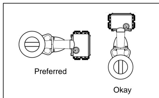
**Configuration for Multi-Fluid Measurement**
